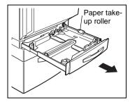
Press down on the paper-lifting plate until it locks into place.
